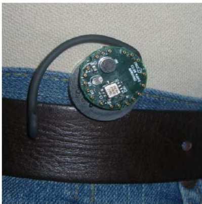
Fig. 15. Wearable sensor that detects anomalous events
